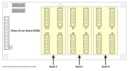
FIGURE 5-2: RELAY DRIVE CONNECTOR BANKS
